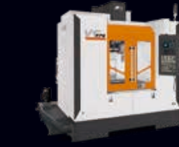
Belt driven spindle up to 10000 rpm Box slideways available
