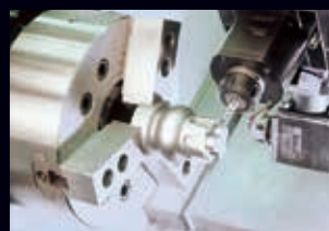
Belt driven spindle available with C axis
